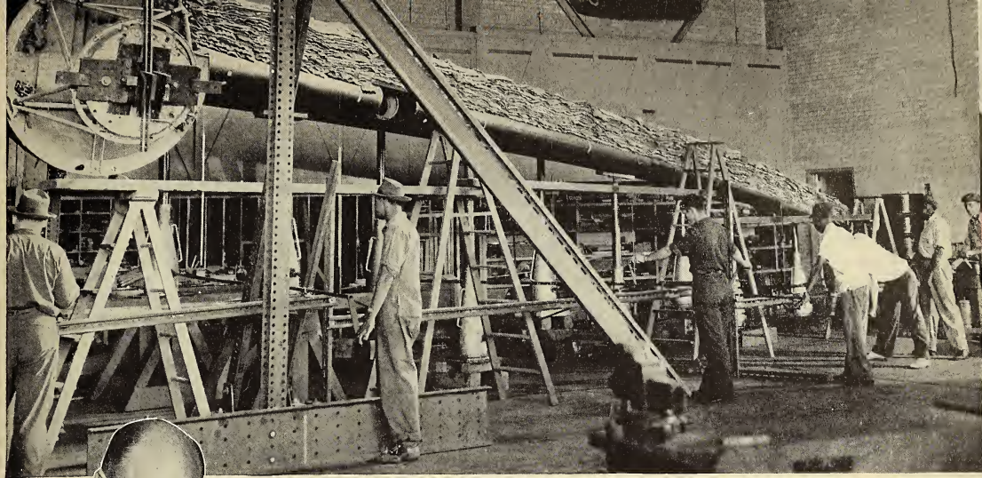
The 10-pound bags on this C-47's wing show how many "Gs" it will take before cracking.
